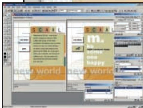
Above: Creating disjoint rollovers – mouseover on the gifts button changes the panel to its right
